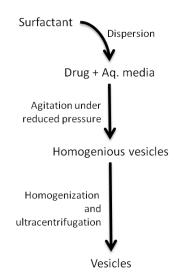
Fig. 3. Preparation of niosomes by aqueous dispersion method
